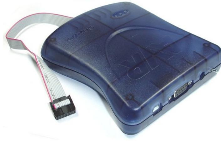
Figure 2: The Atmel JTAG ICE mkII programmer used to download machine code to the AVR Raven and perform in-system debugging via JTAG.
