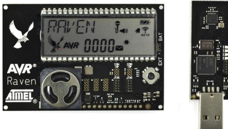
Figure 1: The AVR Raven development board and the RZUSB stick which can be used to access IEEE 802.15.4 based networks.
