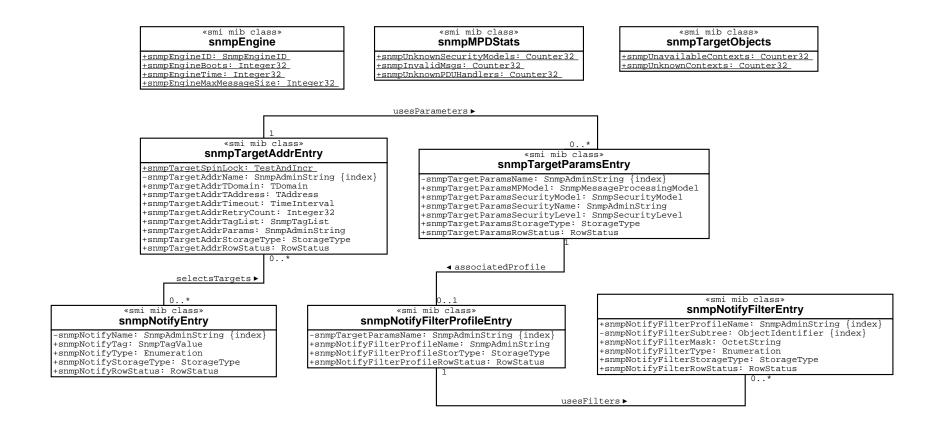
SNMPv3 defines several MIB modules for remote configuration of SNMP entities.
